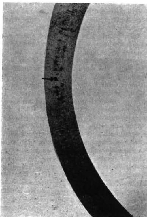
Fig. 2. Part of an X-ray microbeam back-reflexion photograph from an oscillated specimen of heavily rolled aluminium. The arrow indicates diffraction spots with radially displaced central regions. Beam diameter 30 \mu ; 422 reflexion, \text{Cu } K\alpha radiation.
